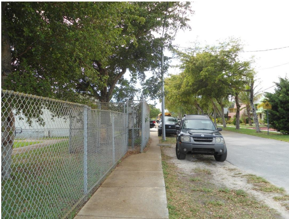
Fence encroaching into the sidewalk (minimum sidewalk width not maintained per ADA requirements)
