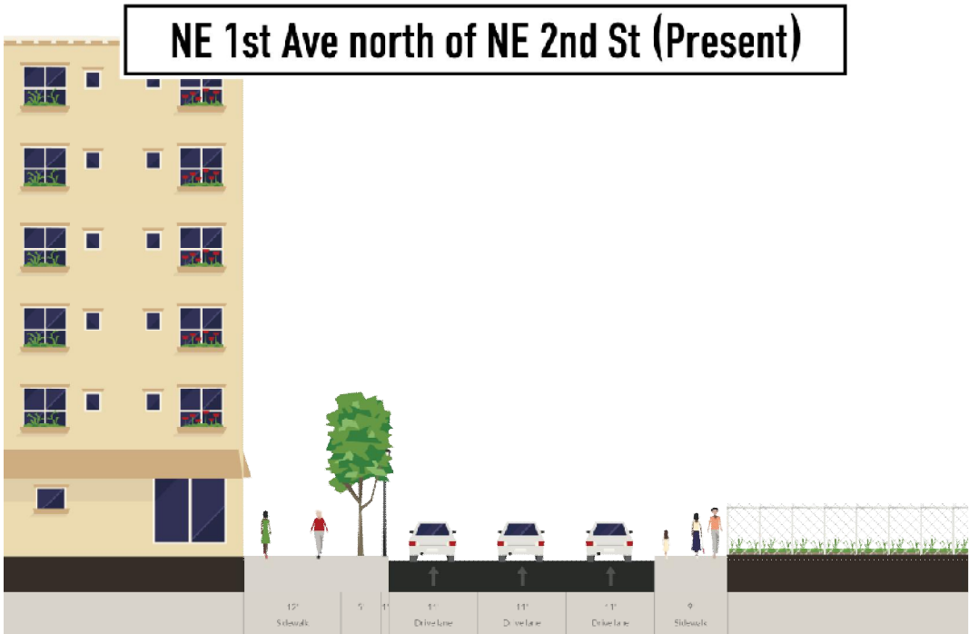
Figure 4-23: Before and After Typical Sections with a BAT lane on NE 1st Avenue
