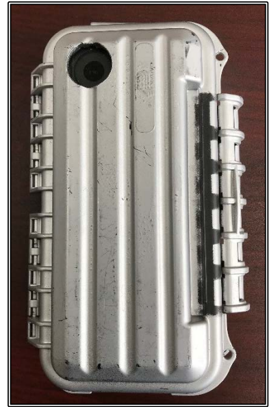
Data collection weatherproof video camera as mounted in silver paint, shown unlocked (all were repainted silver for higher temperature weather)
