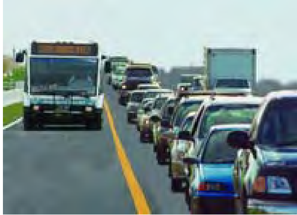
An example of MDT bus on shoulder
