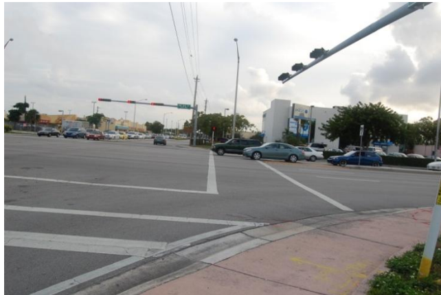
Figure 36: Wide turning radius and Stop line closer to the crosswalk.
