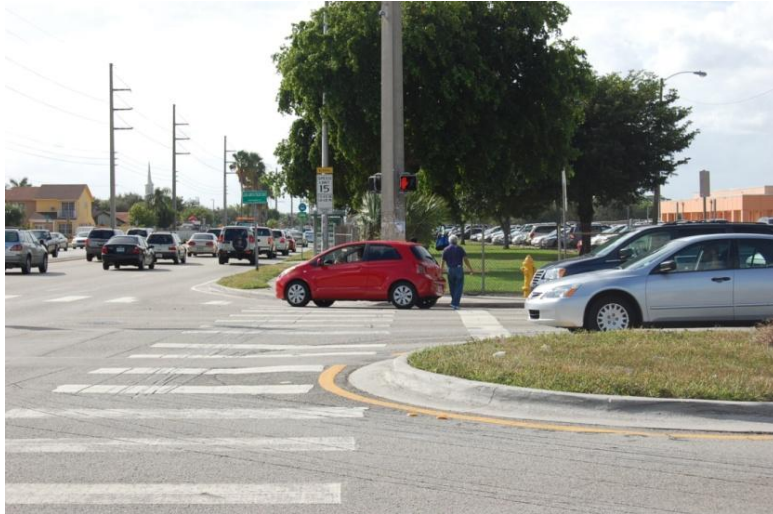
Figure 16 - 17: Pedestrian and right turning vehicle conflict on the crosswalk
