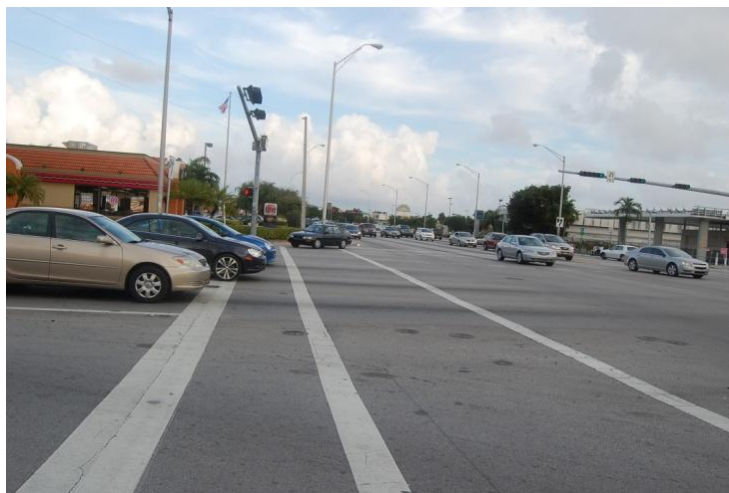
Figure 37: Short clearance distance between crosswalk and stop line
