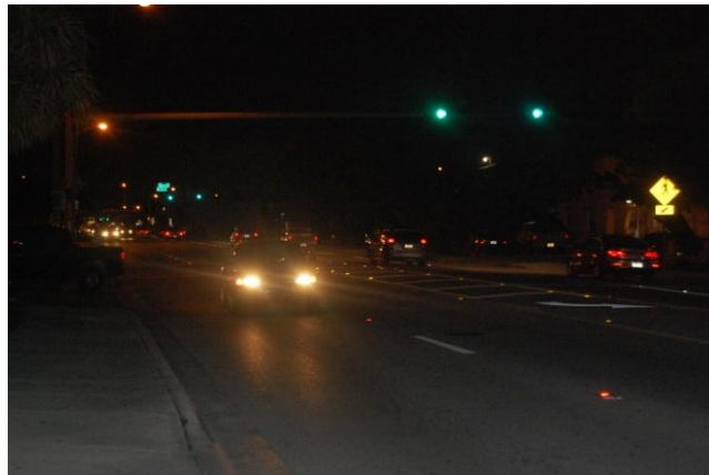
Figure 81: Improper lighting condition at the intersection
