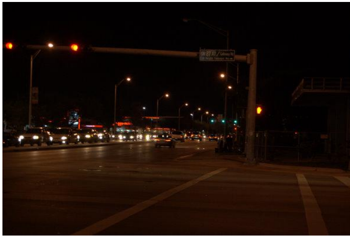
Figure 39: Lacks sufficient lighting on crosswalks at SW 87 th Ave and SW 24 th St (Coral way)
