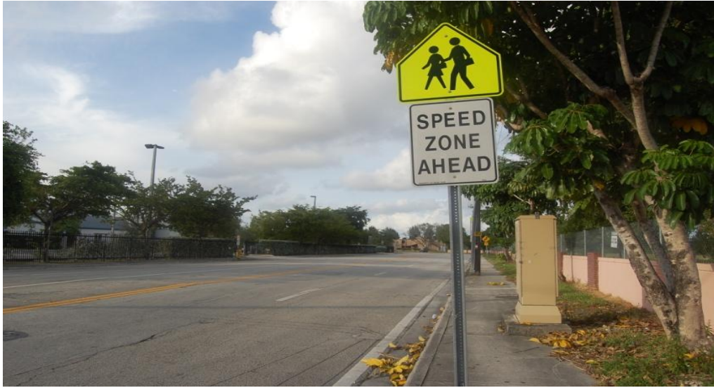
Figure 30: Obstruction along sidewalk – Forces pedestrians to walk on the pavement
