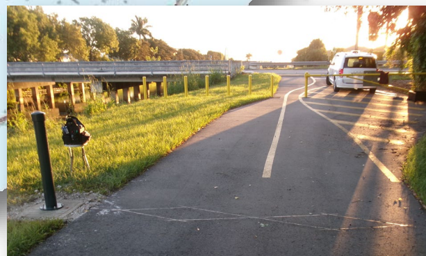
Biscayne-Everglades Greenway, Homestead, Miami-Dade County Side Fire Infrared with Inductive Loops 2023 Avg. Daily Users: 79
