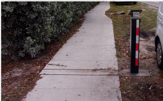
US-1 Overseas Heritage Trail, Key West, Monroe County Overhead + side fire Infrared with piezo-electric sensors Sensors issues throughout 2023* (dual site)
