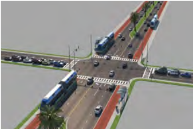
Business Access & Transit (BAT) Lanes
