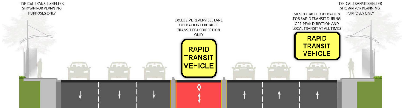
Figure 16 – Reversible Center Lane for Rapid Transit, Source: FDOT-D6 PD&E Study
