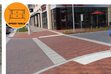
Speed table Improves safety of crossing
