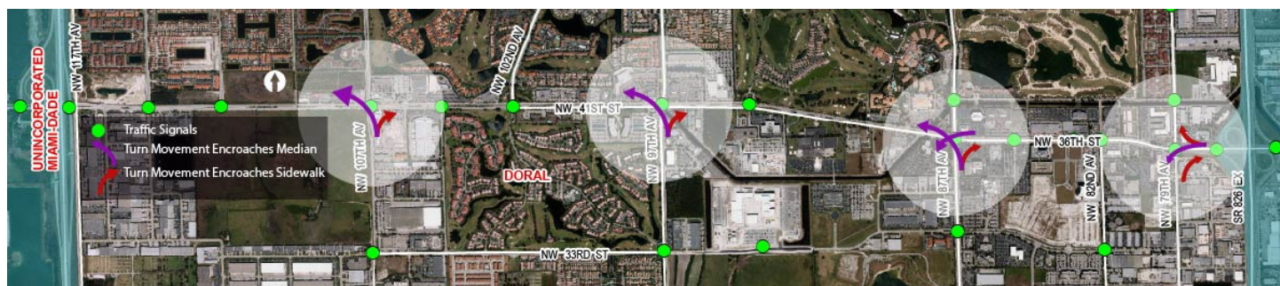
FIGURE 51: DORAL BOULEVARD – INTERSECTIONS WITH TIGHT TURNING RADII FOR HEAVY VEHICLES
