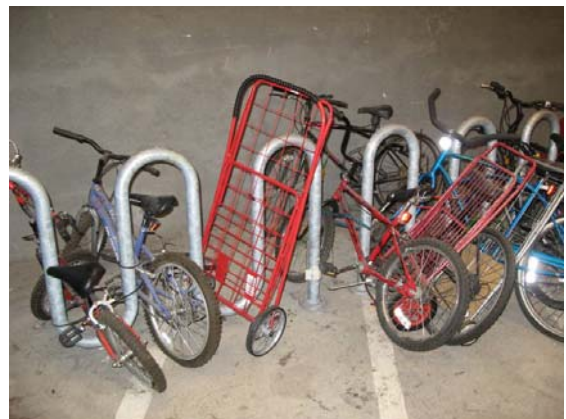
Flawed Rack Design Leading to Improvised Parking
