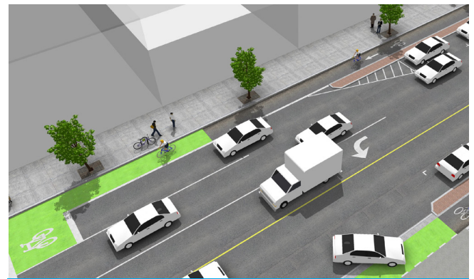
Cycle Track to Bicycle Lane and Bicycle Box
