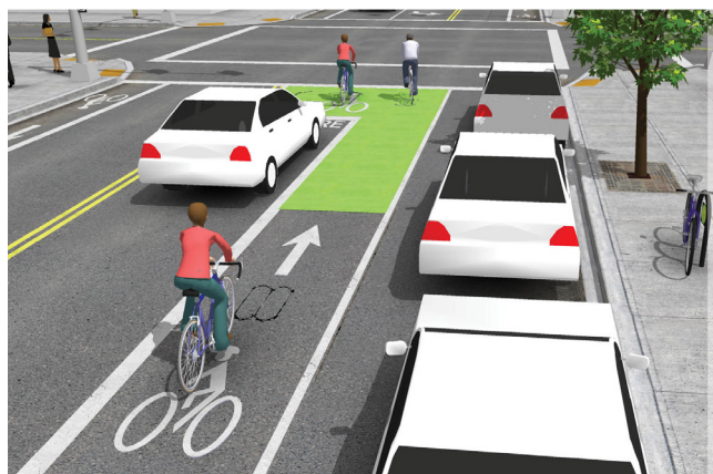
Signal Detection in Bicycle Lane
