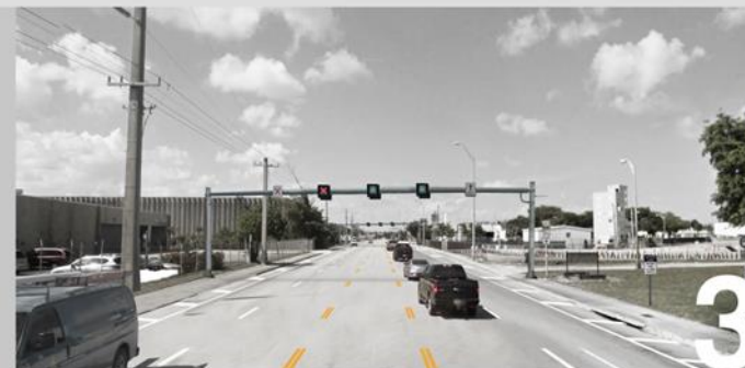
NORTHERN CONDITIONS FROM 103RD STREET TO 119TH STREET UTILIZES PAVED SHOULDERS TO ACCOUNT FOR A WIDER ROADWAY SECTION
