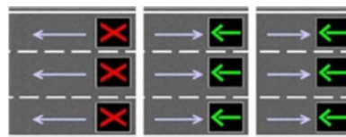
Figure 1: Unidirectional Reversible Roadway Concept
